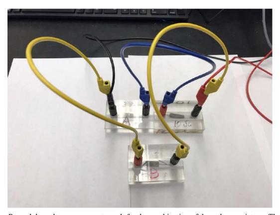
Record the voltage vs. current graph for the combination of these three resistors. The computer will collect data points just as it did in *Activity 2*. On the data sheet, record the slope of this graph, i.e., the total resistance for this combination of resistors. You may now disassemble your circuit. Exit Capstone application.
