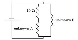
You should try to set up this circuit yourself. However, if you need a little help, you may refer to the diagram below. In fact, it is a combination of resistors in parallel and in series.
